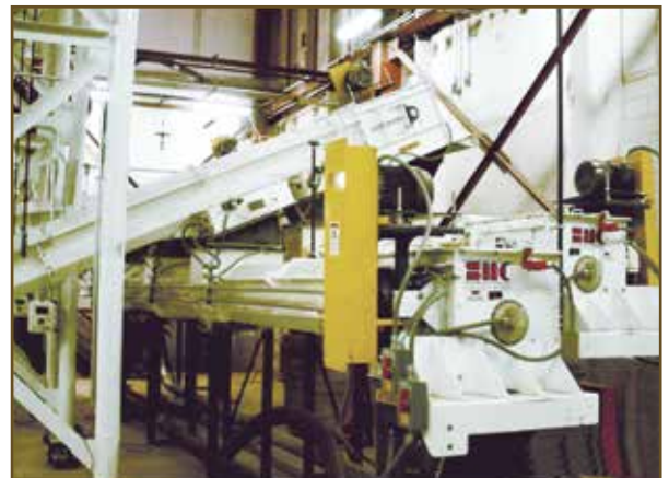
Installation of 3 -16SWR-PF. The conveyors are moving pet food to the bagging operation.
